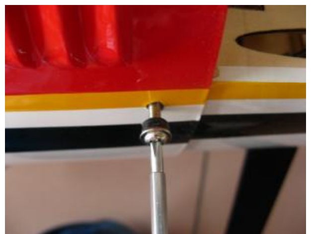
10. Canopy and cowling with shockproof silicon rubber blanket
