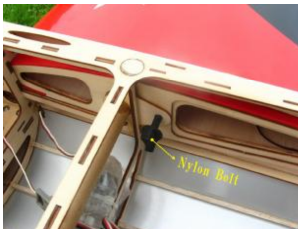
11. Two pieces of removable wings fitted nylon bolt
