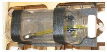
(Here is an example of proper strap location. Note the foam protecting the tank from the wooden tray)
