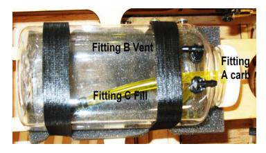
Notice the 90 degree fittings are orientated for optimum vent and fill fuel line routing. To prevent fuel siphoning out the vent line loops to the back of the tank and then out of the fuselage. This will keep the fuel from running out the vent on long down lines.
