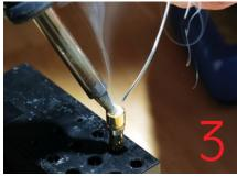
Next, I applied solder to the ends of the EC5 connectors. This is where the soldering helper comes in handy. With the connector firmly placed in the holder, apply heat to the outside of the connector and apply solder to the inside. Fill the connector about half way with solder.
