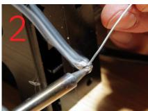
You begin by stripping about 3/16-inch of casing from the ends of the wires. I precut my wires to four inches each (three required total). Then I tinned the wires by applying heat to the bare wire and applying enough solder to coat the entire copper end. Don't apply too much; you should still be able to see all the strands of wire, they will just be silver now instead of copper.
